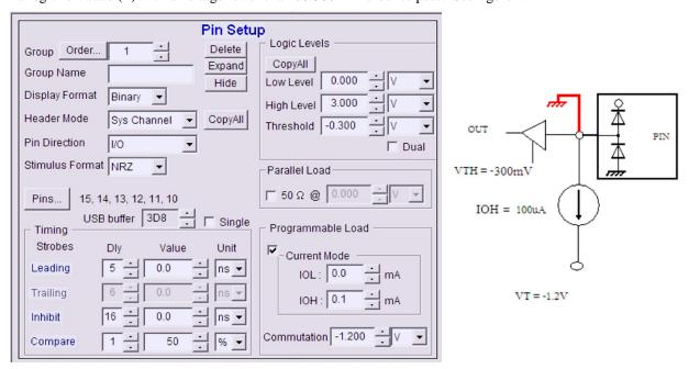
Figure 2: Shorts Test Pin Setup
