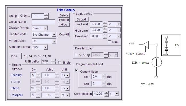
Figure 5: Opens Test Pin Setup
