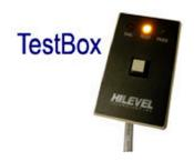
Upon entering the **TestBox** window, we load the ATX file, which loads all vector files into the tester memory. Sub-tests using the same vector files will share the vector space in the tester memory. The obvious benefit of this mechanism is that we don¢t need to download vector files from disk during execution of the test, resulting in extremely fast deployment of multiple vector files.
