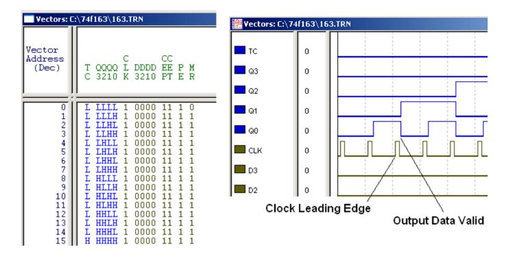
The 74F163 performs its functions on the leading edge of the clock. But some chips may also operate on the trailing edge, or both edges. Clearly the control of both leading and trailing edges on certain pins is crucial for timing measurements.
