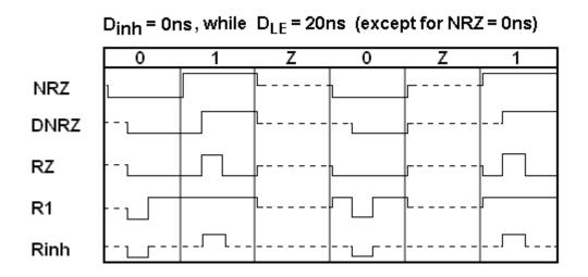
Here we see that setting Inhibit Delay to zero nanoseconds insures that the tester driver will be tristated for the *entire* vector when a "Z" appears as vector data. Most applications perform correctly when this practiced is used. Consequently, HiLevel recommends this approach for new users, applications, or as a starting point whenever you are unsure about the issue.
