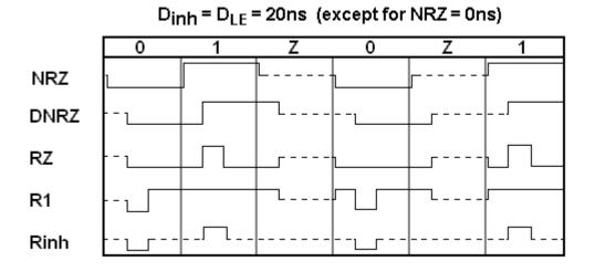
In the first example, we see that vector data continues to be asserted until the inhibit time occurs (which is set to the same delay value as the leading edge). This mode is not recommended unless you have some particular reason for stimulus data to be active during some portion of the cycles (vectors) in which a "Z" appears as the data.
