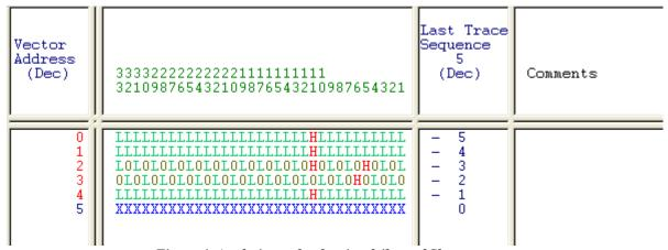
Figure 4: Analysis results showing failure of Shorts test
